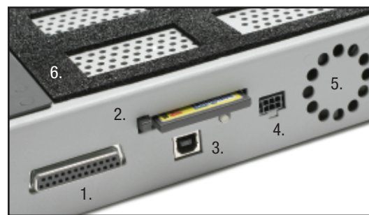
(1) Printer Port, (2) CompactFlash™, (3) USB, (4) Light stack, (5) forced air exit, (6) forced air entrance
